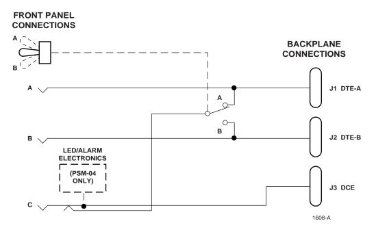
Figure 2-2. PatchSwitch with Off-Line Access (PSM-04, PSM-05)
